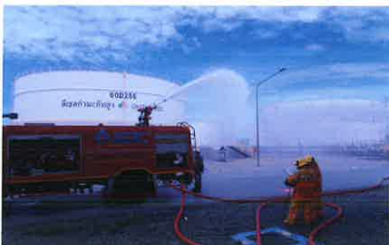
Fire truck discharge cooling shell side of 60D256
